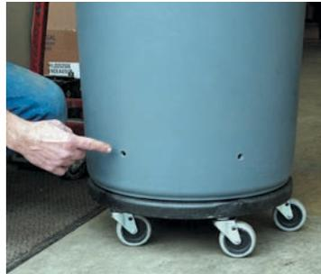
*Drill holes in the sides or bottom of the container*
